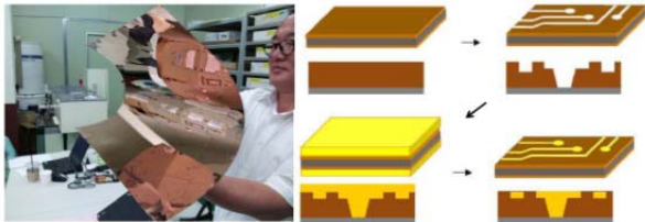
Fig.4 Thin flexible package substrate (left) and its process flow including laser trenching, Cu plating and CMP (right)
