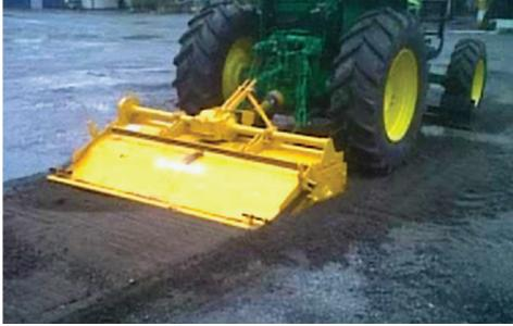
Unimix increases soil stability and strength by uniformly mixing fine and coarse materials throughout the entire mixing depth.
