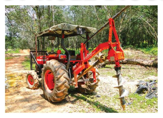
HOWARD's Post-Hole Diggers are labour-saving implements for erecting masts, poles, signs, fences and are increasingly used in tree-crop replanting programmes. Seedlings grown in planting bags in nurseries are transplanted into pre-bored holes, with speed and accuracy.
