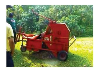
HOWARD's Grass Sweeper HSW collects grass clippings, leaves, twigs etc. into a steel hopper, which can be neatly emptied from the tractor seat.
