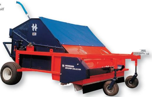
Four rows of easily changeable polybrush combs are fitted horizontally onto a rotor shaft. Wide profile rear turf tyres - and pneumatic front castor wheels which also serve as height adjusters. Designed for sweeping and collecting light debris off uneven terrain - primarily turf, but works equally well on hard surfaces such as running tracks, dirtroads and parking lots, where, however, more bristle wear must be anticipated.
