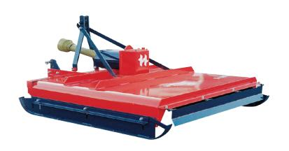
As a general rule, this machine will deal effectively with any jungle undergrowth which a tractor can ride over. HS 44 is also widely used for stubble shaving, ratooning and mulching of fibrous crops such as sugarcane and pineapple. Chain slashing Heads and Disc Stubble Shaver available as optional.
