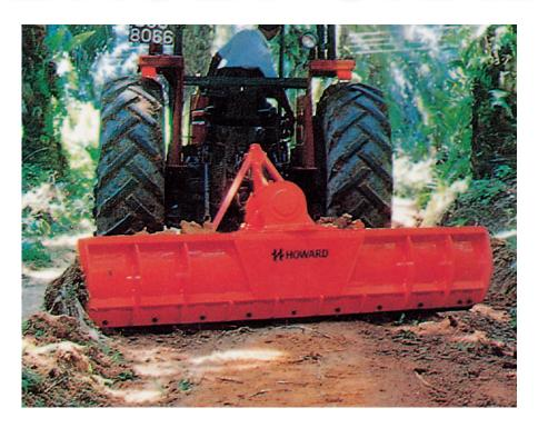
HMG is a heavy-duty rear mounted grader, designed with multiple features such as vertical tilt for ditching; multiset locking 15°-30-45° L/R, and off-set positioning on both sides of the tractor. HMG can swivel 360° and can as such also be set for reverse levelling.
