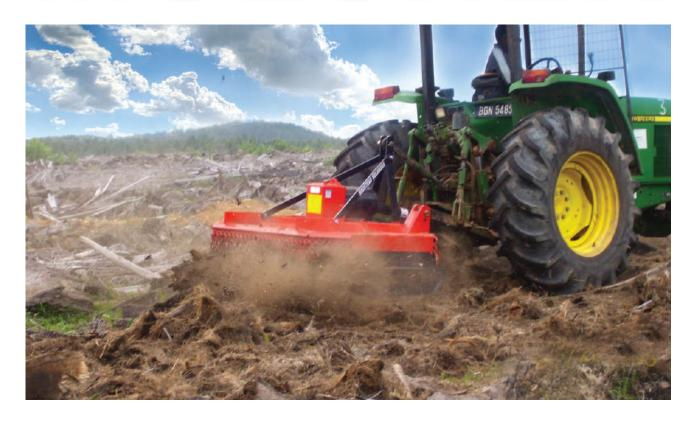
HOWARD has developed a tractor- mounted mechanical shredder, which turns felled tree trunks (chipped) into useful compost.
