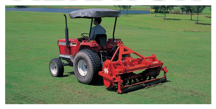
Aerating of turf areas, grassland and fields - is becoming increasingly vital, to overcome the hardpan caused by vehicle and human traffic which otherwise inhibits healthy growth, moisture penetration and fertiliser uptake.
