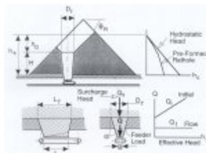
Figure 26: Gravity Reclaim Stockpile
