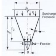
Figure 5. Pressures Acting in Hopper and Feeder
