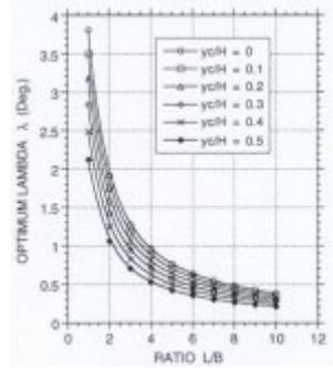
Figure 16. Optimum Divergence Angle versus L/B Ratio for a Range of Clearance Ratios  $\eta_v = 0.75$ ;  $C_e = 0.5$
