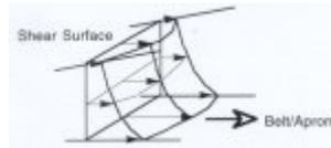
Figure 12. Velocity Profile in Shear Zone
