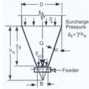
Figure 8 - Loads on Feeder
