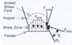
Figure 9. Stress Fields at Hopper and Feeder Interface
