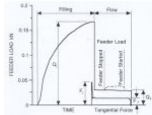
Figure 4. Feeder loads for Belt Feeder Test Rig
