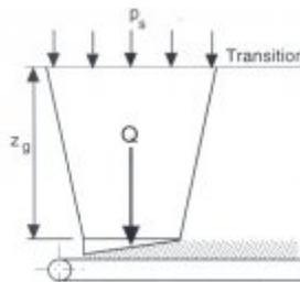
Figure 3. Feeder Loads in Hopper/Feeder Combination
