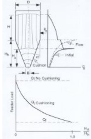
Figure 22. Cushioning in the Hopper to Control Feeder Loads
