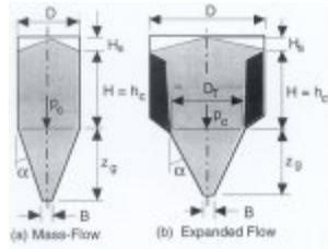
Figure 25. Mass-Flow and Expanded-Flow Bins
