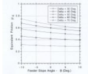
Figure 19. Equivalent Friction for Belt and Apron Feeder -  $\psi = 10^\circ$
