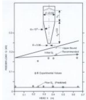
Figure 10: Comparison between Predicted and Experimental Results - Feeder Test Rig Bulk Material: Plastic Pellets
