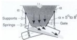
Figure 2: Vibratory Feeder
