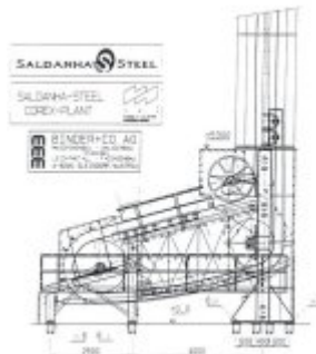
Figure 6. Bottom station of the vertical conveyor
